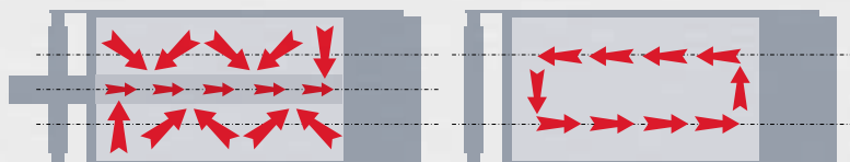
Weiler® twin overlapping, counter-rotating paddle system with unload screw.
